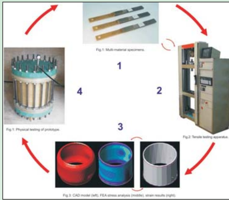
Design cycle using virtual and physical prototyping.
